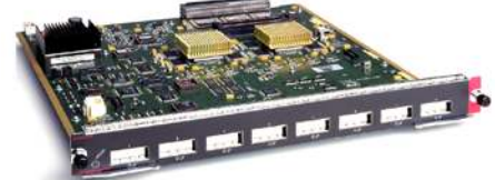
8 Port GBIC-Based Module
