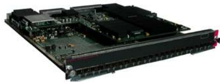
24 Port SFP-Based Module
