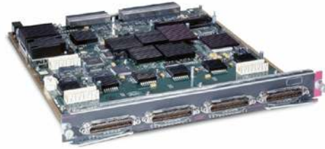
Figure 4. Cisco Express Forwarding 256 Copper 10/100 Interface Module (part number WS-X6548-RJ-21)
