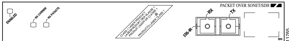
Figure 1-3 PA-POS-OC3SMI—Faceplate View, Horizontal Orientation
