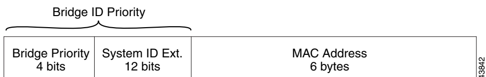
Figure 7-9 Bridge Identifier with MAC Address Reduction Enabled
