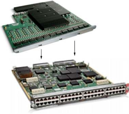
Figure 7. Cisco Classic 96-Port 10/100 802.3af PoE Module (part number WS-X6148X2-45AF)
