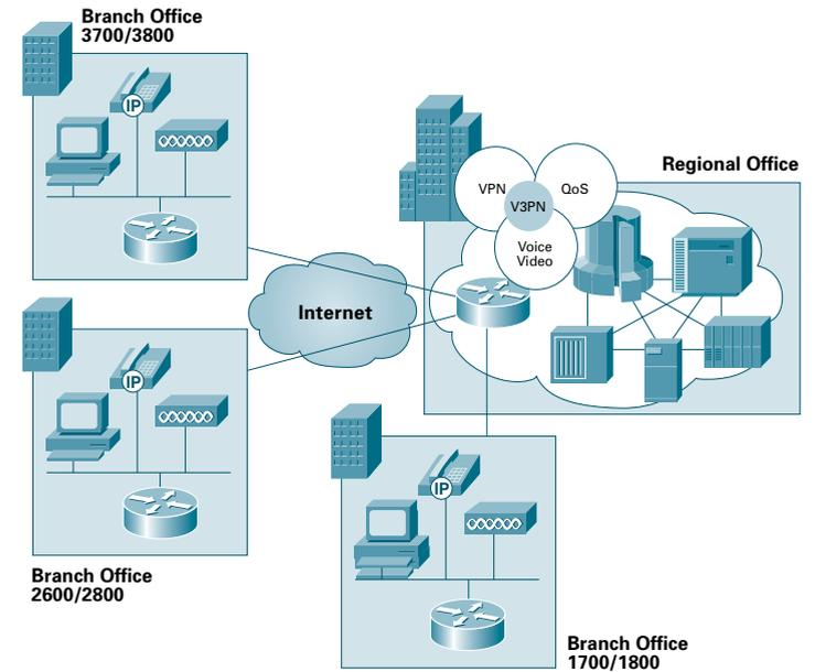
The figure above shows the Cisco 3800 Series routers converge voice, video, and data across a secure IPSec VPN network with high-quality, reliable performance. DMVPN creates tunnels on-the-fly based on user traffic. V3PN functionality provides QoS, multiprotocol, ease of provisioning, and secure connectivity.
