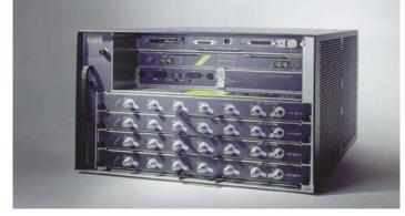
offer varying upstream-to-downstream interface ratios, differing bandwidth, modulation schemes, and the ability to dynamically perform complex spectrum management. The router supports 6 MHz North American channel plans using ITU-T J.83 Annex B operation and 8 MHz Phase Alternate Line (PAL) or Sequential Coulour Avec Memoire (SECAM) channel plans using ITU-T J.83 Annex A operation.
