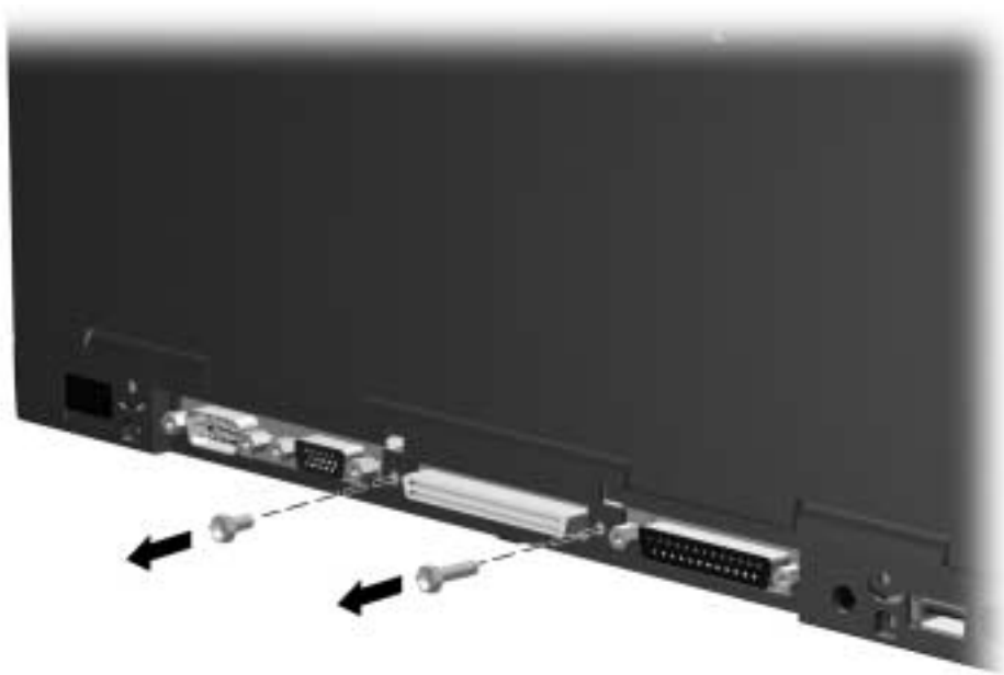
Figure 5-34. Removing the Bushing Guides
