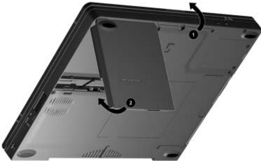
Figure 5-6. Inserting a Battery Pack
