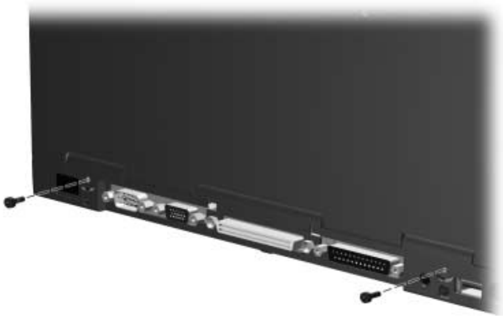
Figure 5-22. Removing the Switch Cover Screws
