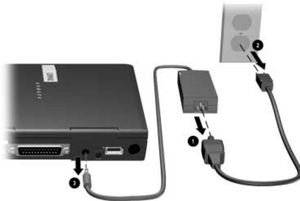
Figure 5-3. Disconnecting the Computer
