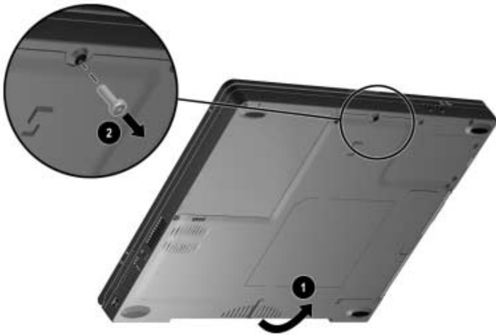
Figure 5-7. Removing the Hard Drive Screw
