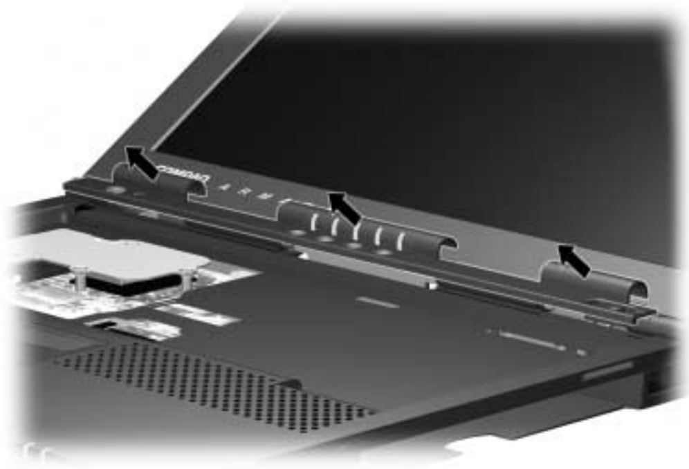
Figure 5-23. Removing the Switch Cover
