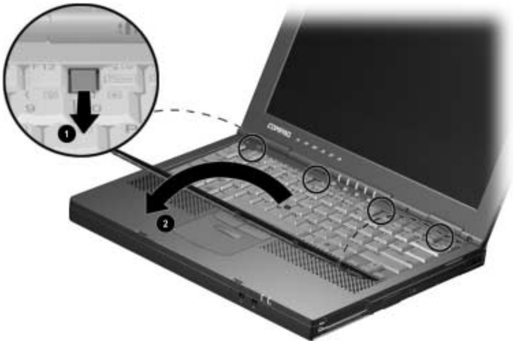
Figure 5-18. Removing the Keyboard
