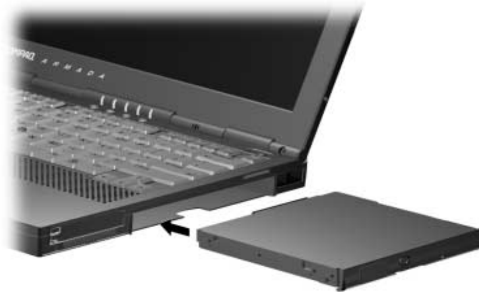
Figure 5-11. Inserting a Device into the MultiBay
