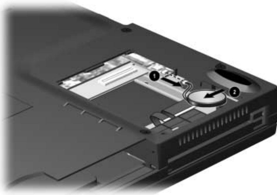
Figure 5-17. Disconnecting the RTC Battery Cable
