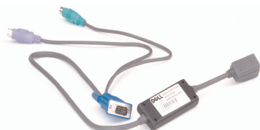
Dell Server Interface Pod (SIP)
