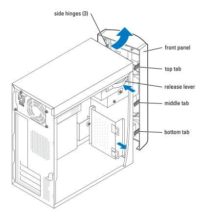
7 Pull the two front-panel tabs towards you, and then push out the front-panel insert.
