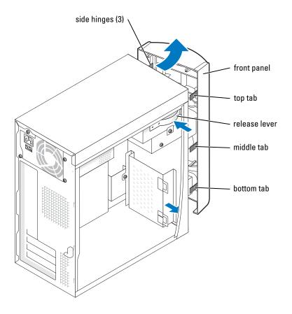
7 Press in the two insert tabs, and then push out the front-panel insert.
