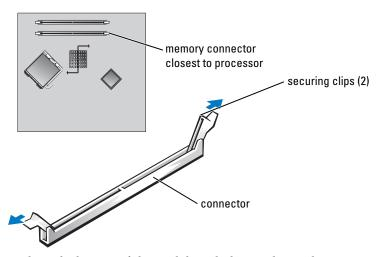
Align the notch on the bottom of the module with the crossbar in the connector.
