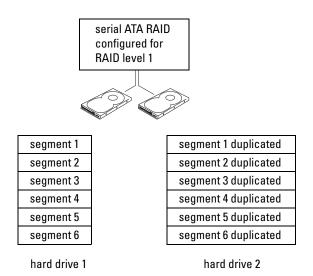
If a drive failure occurs, subsequent read and write operations are directed to the surviving drive. A replacement drive can then be rebuilt using the data from the surviving drive. Also, because data is duplicated on both drives, two 120-GB RAID level 1 drives collectively have a maximum of 120-GB on which to store data.
