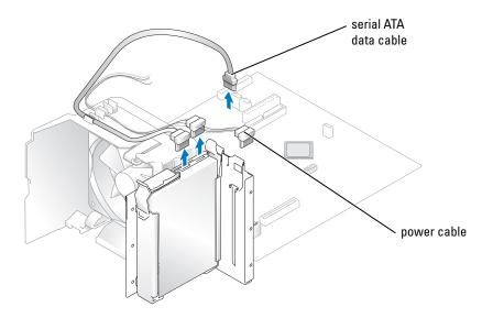
**3** Press in the blue tabs on each side of the drive towards each other and slide the drive up and out of the computer.
