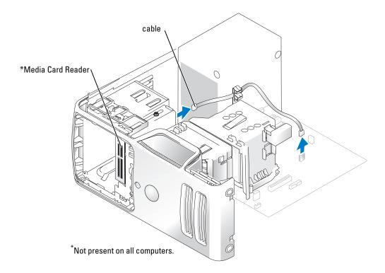
**3** Disconnect the USB cable on the back of the Media Card Reader from the FlexBay USB connector on the system board (see page 65) and route the cable through the clip on the shroud.
