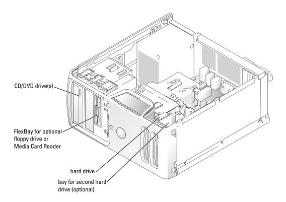
Connect CD/DVD drives to the connector labeled "IDE" on the system board. Serial ATA hard drives should be connected to the connectors labeled "SATA0" or "SATA1" on the system board.
