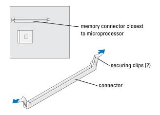
9 Align the notch on the bottom of the module with the crossbar in the connector.
