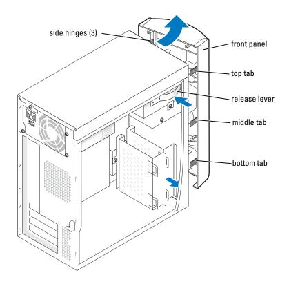
7 Press in the two insert tabs, and then push out the front-panel insert.
