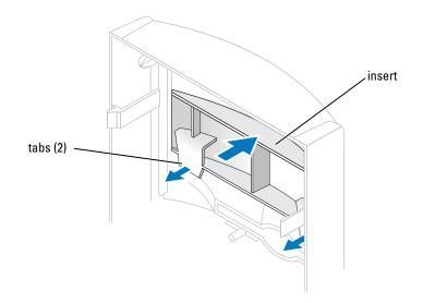
7 Pull the two front-panel tabs towards you, and then push out the front-panel insert.
