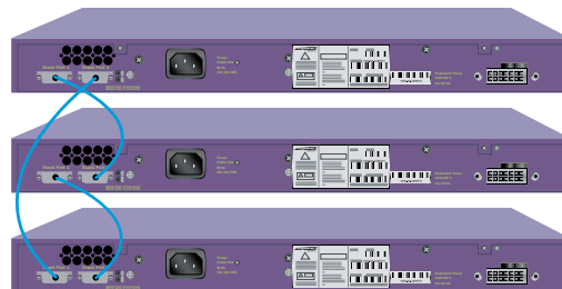
Figure 1: Summit 400-24t UniStack Stack Cabling Illustration
