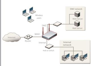
configuration changes. You would typically use the FortiWiFi unit in Transparent mode on a private network behind an existing firewall or behind a router. In its default Transparent mode configuration, the unit functions as a firewall. No traffic can pass through the FortiWiFi unit until you add firewall policies.
