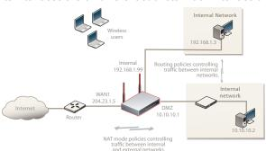
configured with an IP address that is valid for that network. You would typically use NAT/ Route mode when the FortiWiFi unit is deployed as a gateway between private and public networks. In its default NAT/Route mode configuration, the unit functions as a firewall. Firewall policies control communications through the FortiWiFi unit. No traffic can pass through the FortiWiFi unit until you add firewall policies.
