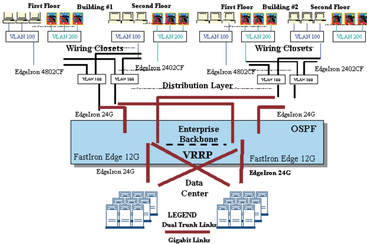
Figure 2.3 illustrates how the FES12GCF fits into the Distribution Layer of the enterprise network.
