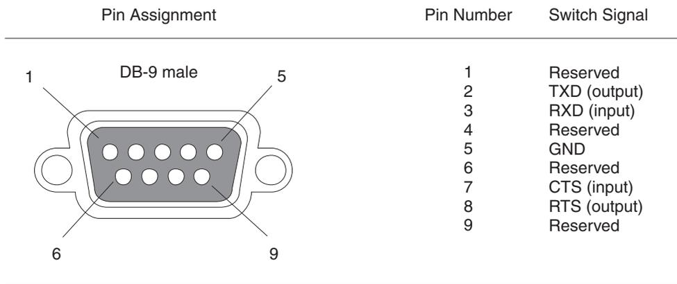
Most PC serial ports require a cable with a female DB-9 connector. However, terminal connections will vary, requiring a cable with either a DB-9 or DB-25 connector, male or female.
