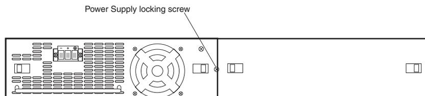
2. If the empty power supply bay has a cover plate, press inward on the two latches near the edges of the cover plate to unlock the plate, then remove the plate.
