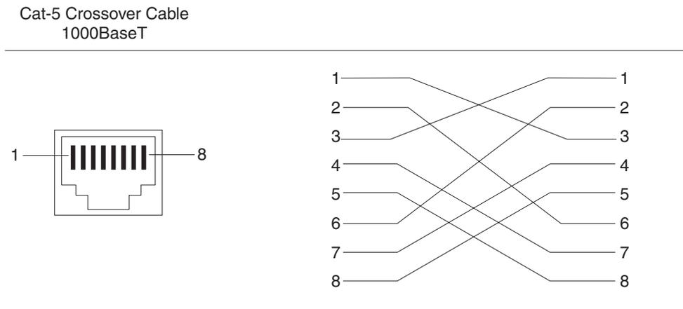
**NOTE:** The 802.3ab standard calls for automatic negotiation of the connection between two 1000BaseT ports. Consequently, a crossover cable may not be required; a straight-through cable may work as well.
