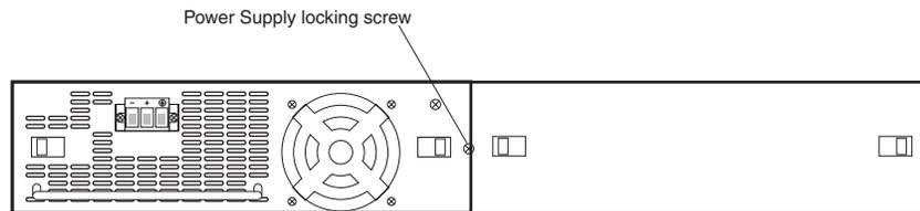
2. If the empty power supply bay has a cover plate, press inward on the two latches near the edges of the cover plate to unlock the plate, then remove the plate.
