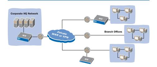
**WX 60:** The WX 60 application acceleration platform, designed for large branch office and small data center applications, features two copper fail-to-wire 10/100/1000 Ethernet ports and supports total reduction throughput speeds ranging from 512 Kbps to 20 Mbps. The WX 60 also supports up to 110 connections to sites where other WX or WXC platforms are installed.
