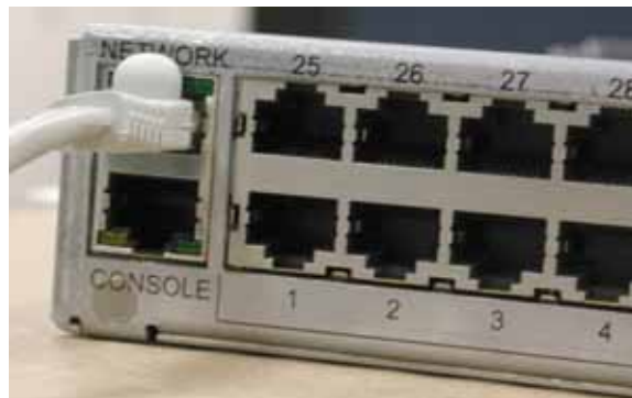
Figure 1-5. SCS4805 Rear Panel Connections for Network, Terminal (Console), and Device Ports
