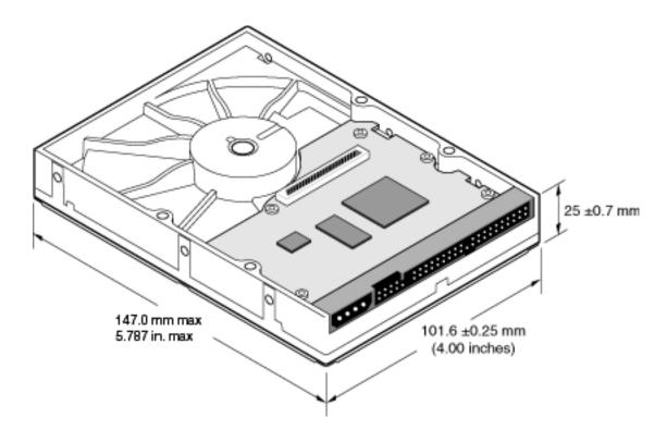
Figure 3-1 Mechanical Dimensions of Maxtor DiamondMax Plus9 Hard Disk Drive
