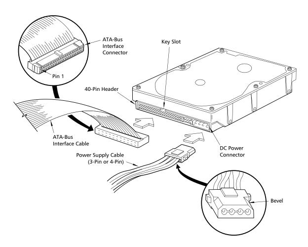
Figure 3-11 Drive Power Supply and ATA Bus Interface Cables
