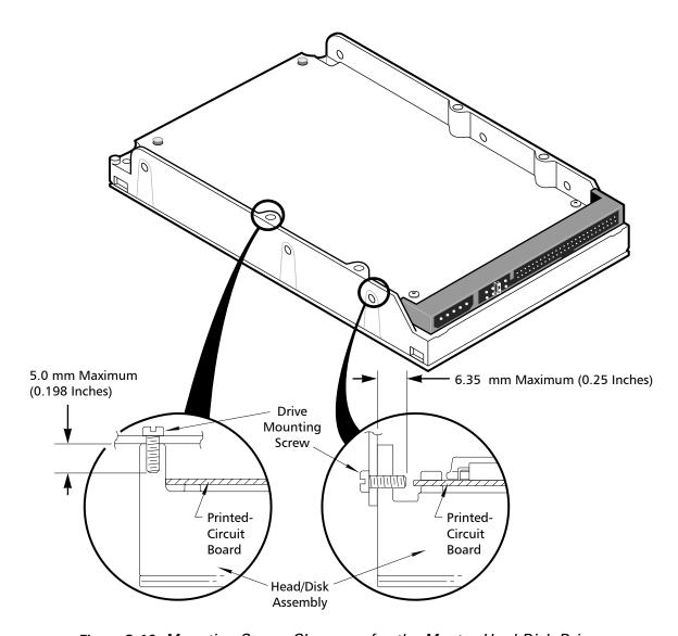
Figure 3-10 Mounting Screw Clearance for the Maxtor Hard Disk Drives
