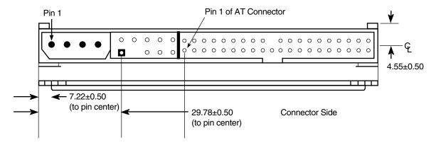
Figure 3-5 AT Connector and Jumper Location
