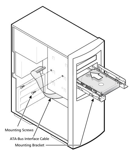
Figure 3-12 Completing the Drive Installation
