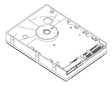
Figure 3-7 The SATA Interface Connector
