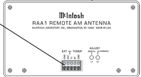
TO MULTIZONE CONTROLLER connects to the McIntosh Multizone Controller Input B
