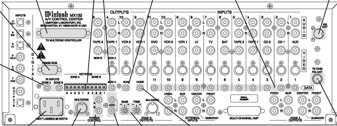
Connect the MX132 power cord to a live AC outlet. Refer to information on the back panel to determine the correct voltage
