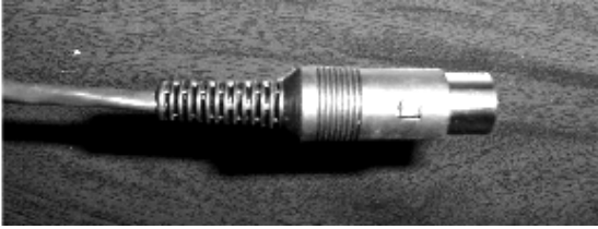
Figure 18. Jacket Placed Over 8-Pin DIN Connector
