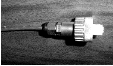
Figure 21. Woodhead Cover Placed Over RJ-45 Connector
