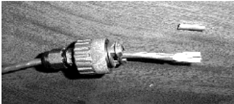
Figure 19. CAT5 Cable with Insulation Removed
