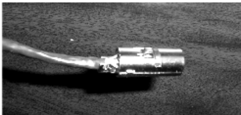
Figure 17. Metal Shell Placed Over 8-Pin DIN Connector
