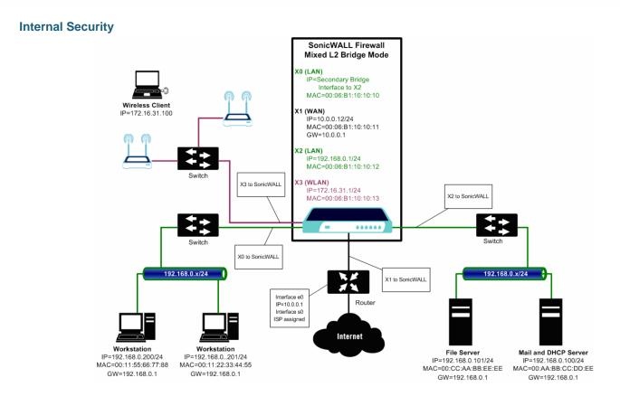
This diagram depicts a network where the SonicWALL will act as the perimeter security device and secure wireless platform. Simultaneously, it will provide L2 Bridge security between the workstation and server segments of the network *without having to readdress any of the workstation or servers*.
