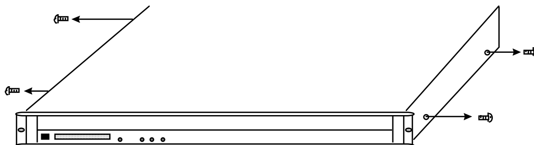
Figure 37 - Removing the Screws Securing the Cover
