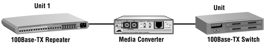
Figure 2 Example of a Duplex Mode Mismatch
