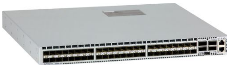
Arista 7050S-64: 48 x 1/10GbE SFP+ and 4 x 40GbE QSFP+ ports
