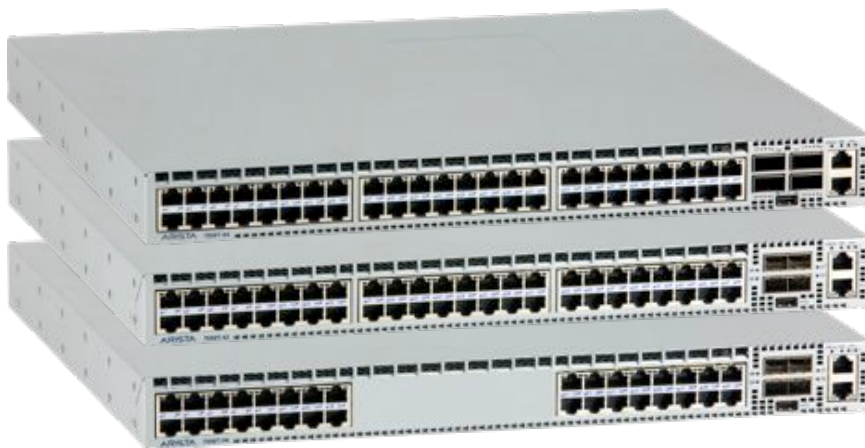
Arista 7050T: 32 or 48 x 1/10GbE BaseT ports and 4 x 1/10GbE SFP+ or 4 x 40GbE QSFP+ ports
