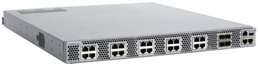
Arista 7120T-4S: 20-port 1/10GBASE-T (RJ-45) + 4 SFP+, 480 Gbps, 360 Mpps, L2/3/4
