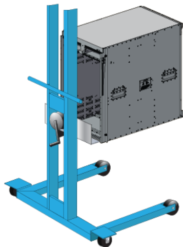
Figure 3-15: Lifting the 12-slot chassis
