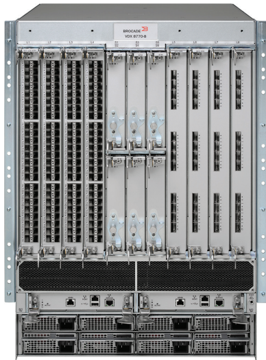
Figure 2: The Brocade VDX 8770-8 Switch supports up to 384 10 GbE ports, 216 40 GbE ports, and 48 100 GbE ports.
