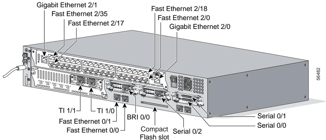
The slot number for all WIC interfaces is always 0. (The W0 and W1 slot designations are for physical slot identification only.) Interfaces in the WICs are numbered from right to left, starting with 0/0 for each interface type, regardless of which physical slot the WICs are installed in. Some examples are as follows:
