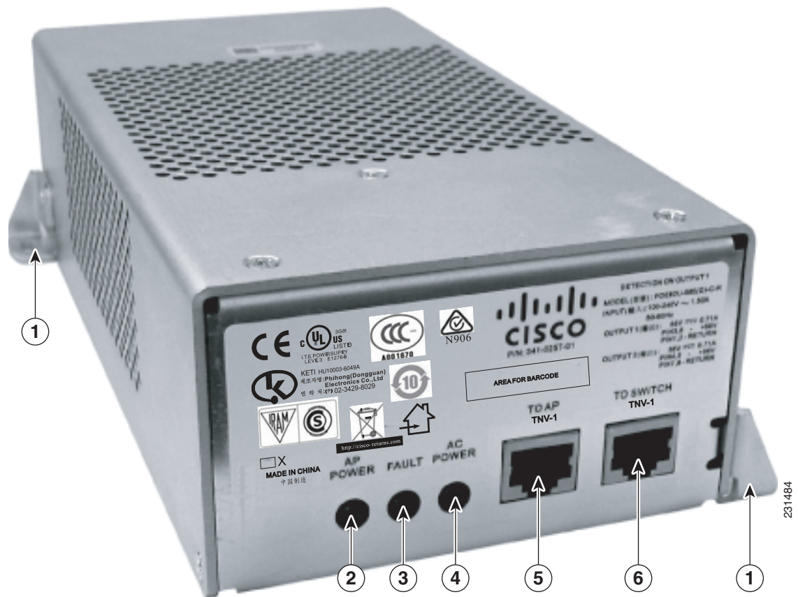
Figure 3-4 Power Injector Connectors and LEDs
