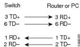
Figure 11: Two Twisted-Pair Crossover Cable Schematic
