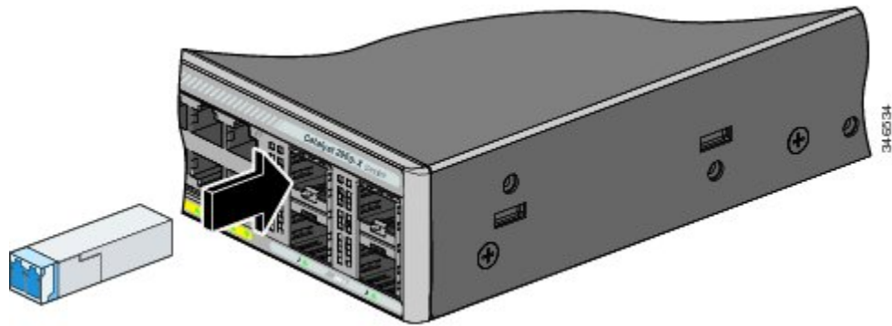
Figure 35: Installing an SFP Module
