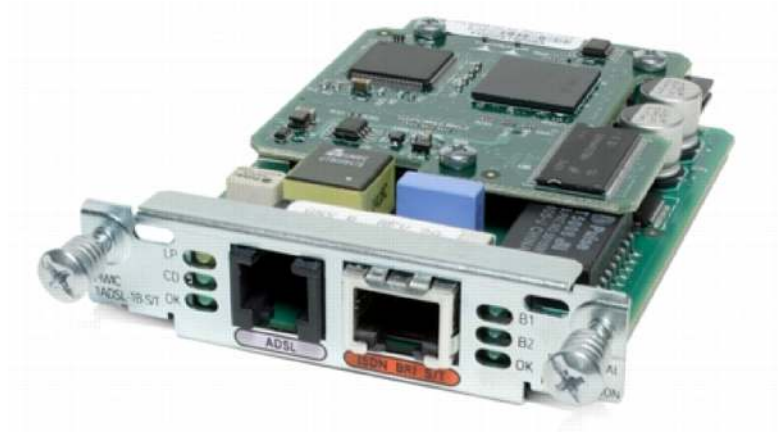
Figure 3. Single-Port HWIC with Annex M (HWIC-1ADSL-M)
