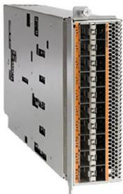
The Cisco Nexus 6004EF also supports a 100 Gigabit Ethernet expansion module that supports 100 Gigabit Ethernet with CXP optics. The 100 Gigabit Ethernet LEM offers four 100-Gbps CXP ports with support for up to 32 ports in a fully loaded system (Figure 4).
