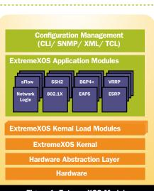
Figure 1: ExtremeXOS Modular Operating System
