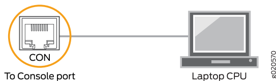
Figure 60: Connecting a Device Directly to a Management Console
