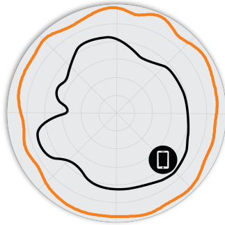
Figure 3. R650 5GHz Azimuth Antenna Patterns
